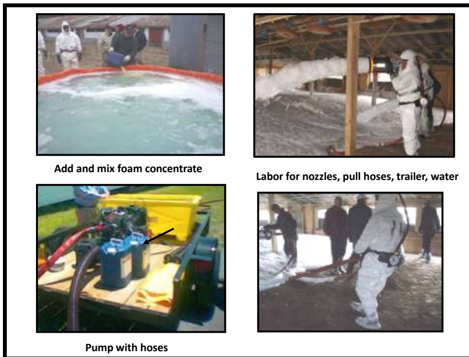
Figure 1. Nozzle system for mass depopulation using water-base foam.
