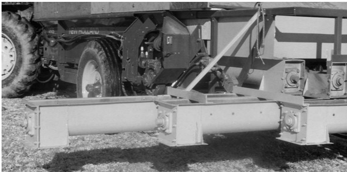
Figure 1. (a) schematic diagram of a solid waste topdresser, and (b) a photograph of the left side of the topdresser used in this study.
