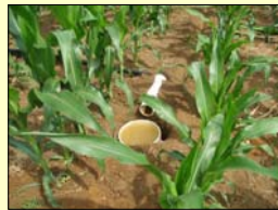
Fig. 3: Sampling device at downslope edge of the plots to collect surface runoff samples.
