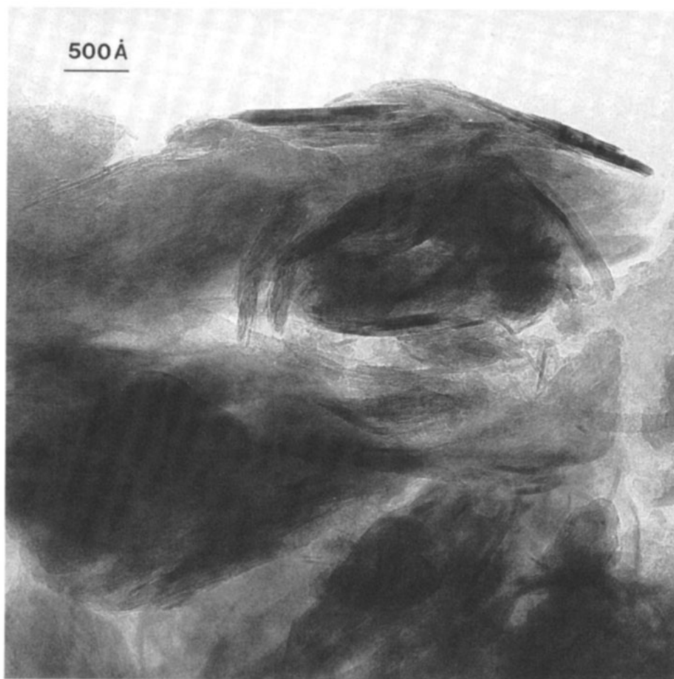
Fig. 4. Low-magnification transmission electron microscope image of unreacted pyrophyllite, showing plate- and needle-like structures characteristic of this material. Note the absence of any visible surface deposits.
